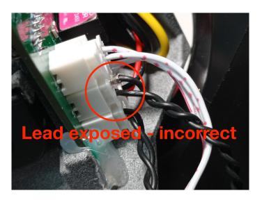
5) To fix the faulty connector, remove it from the socket and push the pin fully into the connector housing. Then re-seat the connector.
